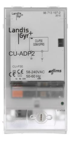
The E65C CU adapter CU-ADP2 permits the external operation of Landis+Gyr communication units (from 2<sup>nd</sup> generation onwards) together with meters, in which no communication unit can be fitted. It generates the supply voltage for the built-in communication unit from the mains voltage.
